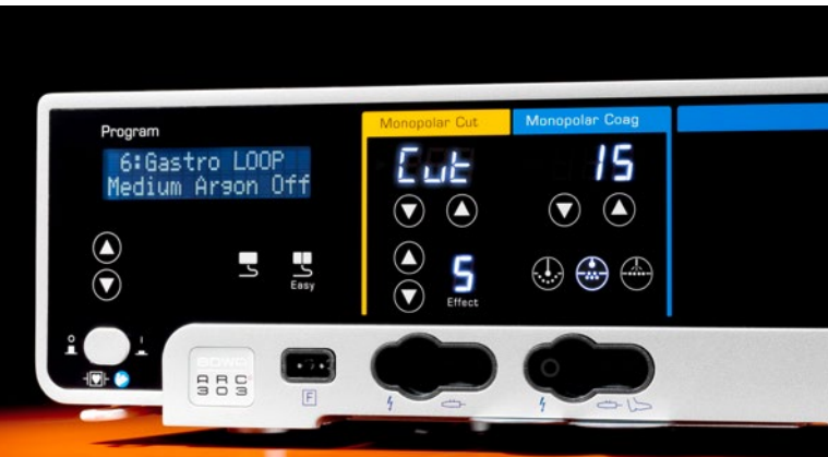
GastroCut offers protection against perforation with polypectomies, papillotomies or endoscopic resections with loops or needle electrodes
