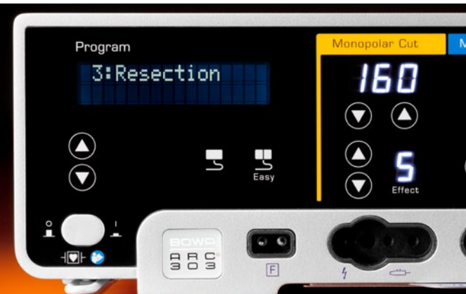
The resection program allows for the use of 300 W for vaporisation with monopolar resectoscopes
