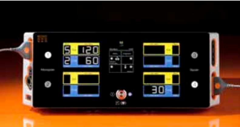
Clarity: Every connected socket – in this photo the upper left and lower right – is clearly assigned to one quadrant of the display
