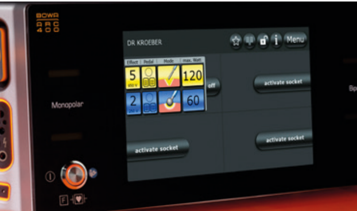
Plug'n Cut: The ARC 400 automatically detects that a standard instrument is connected
